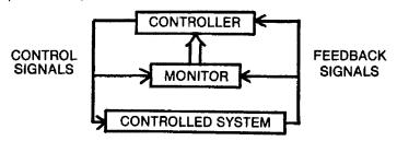
If we left out the monitor we would have a simple cybernetic system. By placing the monitor in the system, the monitor can observe system performance and send information to the controller for changing the performance of the system.
